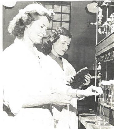
Bernice Galletly and Kathleen Killoran, two Chemistry graduates from the University of Toronto, test buna-S rubber with acetone at the Polymer Rubber Corporation in Sarnia, Ontario.
